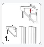
Identify the Vertical Rail, Horizontal Rail, and Pivoting Bracket. Loosen the screws on the Pivoting Bracket slightly-just enough to allow the rails to slide into place.
