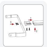
Insert the Rear Tilt Adapter into the front of the Horizontal Rail and secure it with the two small Cap Screws. Then, attach the Rear Tilt Bracket using the included Flat Head Screws.
