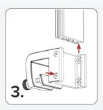
Loosen the screws on the Aquarium Mounting Clamp. Slide the clamp onto the Vertical Rail and position it at the desired height for the HMS mount above the aquarium.
