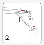
Insert the Horizontal and Vertical Rails into the Pivoting Bracket as shown above. Tighten the screws on the pivoting bracket to temporarily secure the rails in place.
