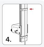
Use the HMS Clips to run the cable along the HMS, ensuring you create a drip loop. Insert the HMS AI End Caps, if desired.
