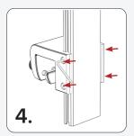
Using the included Hex Key, tighten the screws on both sides of the clamp to secure it in place. Note: Height can be adjusted later by loosening these screws.
