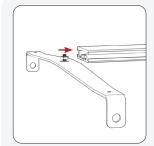
Insert a Flat Head Screw into the Top Tilt Bracket. Loosely attach the Washer and Nut. then insert the Nut into the Horizontal Rail. Position as desired and tighten to secure.
