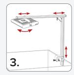
With the HMS secured, adjust the rails and bracket for height, depth, and angle. Loosen screws to adjust, then re-tighten. Note: Two people may be needed
