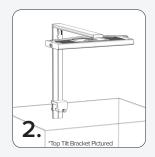
Place the assembly onto the edge of the aquarium at the desired mounting location.
