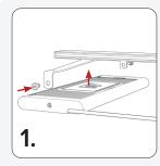
Attach the light to the Tilt Bracket using the included Mounting Screws. Note: Ensure the power cord is positioned toward the back.
